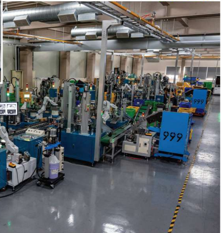
Robotized 2-component injection molding
